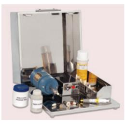
Each punch tip is formed to a very high degree of accuracy and a slight wear & tear can result in production of excessively dull or collared tablet. Polishing of punch cavity is an important exercise to ensure reliability of the tableting process. The punch cavity polishing kit helps you in acquiring the original cavity finish of your punches. There kit contains different types of brushes for different cavities & different types of pastes for varied application.
