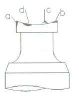
The 4 most common errors in punch cavity polishing are :
